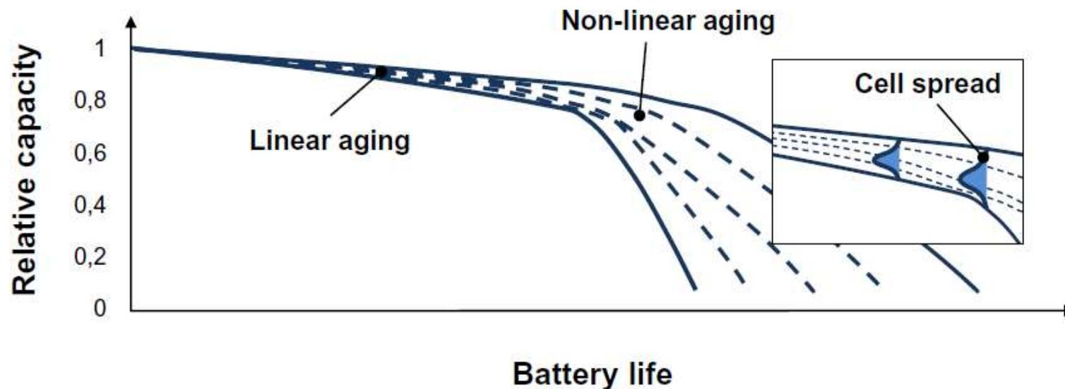
Single cells undergo an **unbalanced electrochemical degradation over time** (Rohr et al., 2017). When the automotive pack is retired, each cell has a unique state-of-health.
